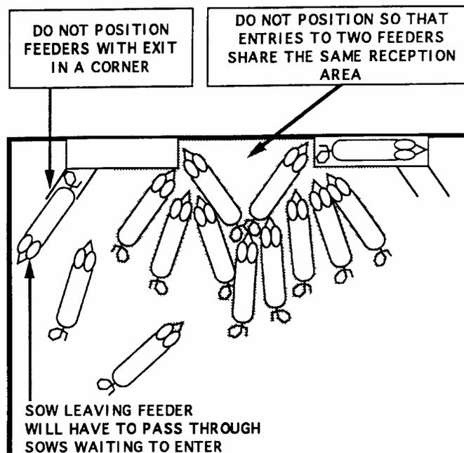
**Figure 5. Avoid positioning feeders such that sows exiting from one feeder impede sows entering another.**
